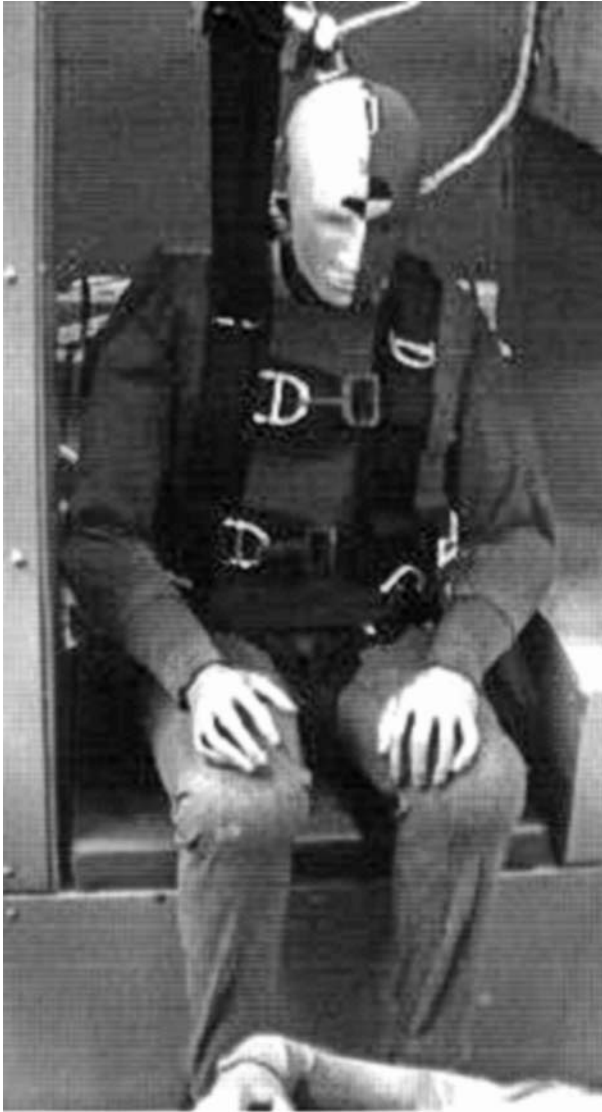
Figure 3. System A, three ambulance mounted tethers and retractors with lap belt (pretest).
