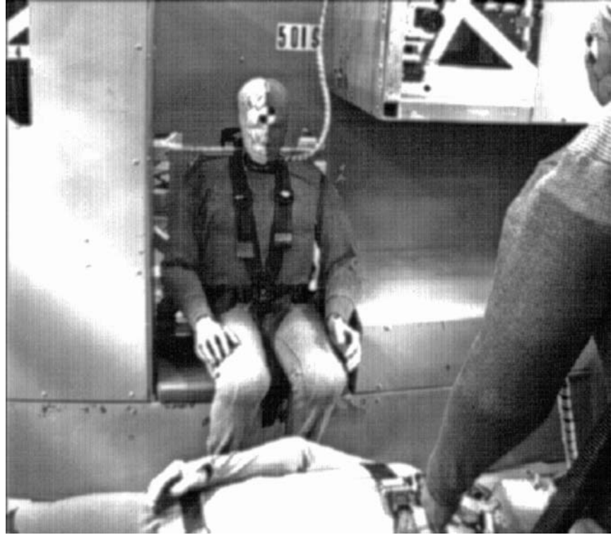
Figure 5. System C (pretest), three-tether harness with web- and vehicle-sensing retractors.
