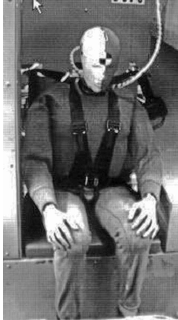
Figure 4. System B (pretest), four-tether harness.
