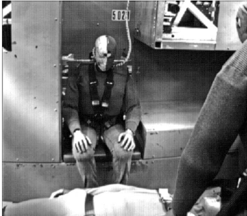
Figure 6. System D (pretest), three-tether harness with web-sensing retractors.
