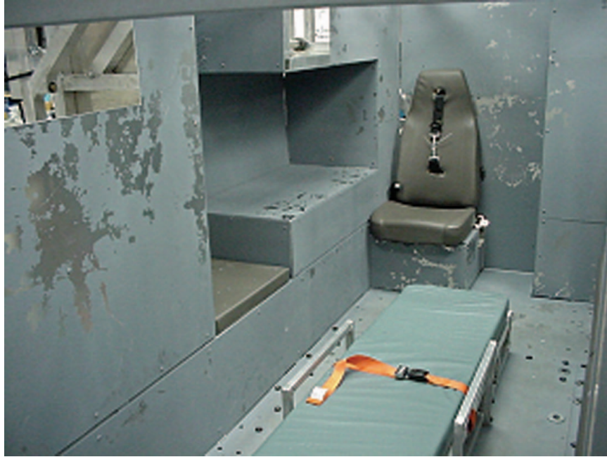
Figure 7. Interior of patient compartment buck looking in from rear doorway, street side.
