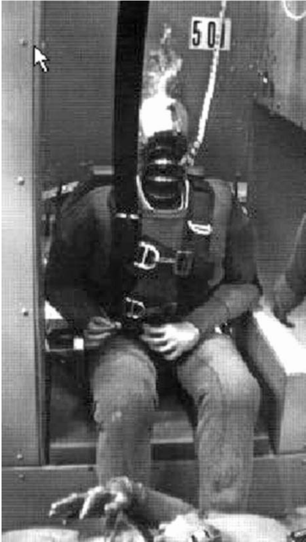
Figure 10. CPR seated ATD viewed from the right side of the patient compartment, side impact test with head-to-wall contact.
