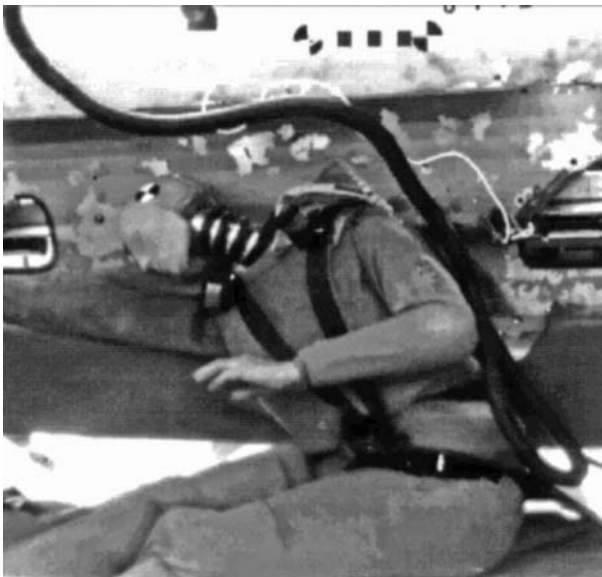
Figure 2. Seated side-facing ATD in five-point restraint at maximum excursion during 40-km/h frontal impact.
